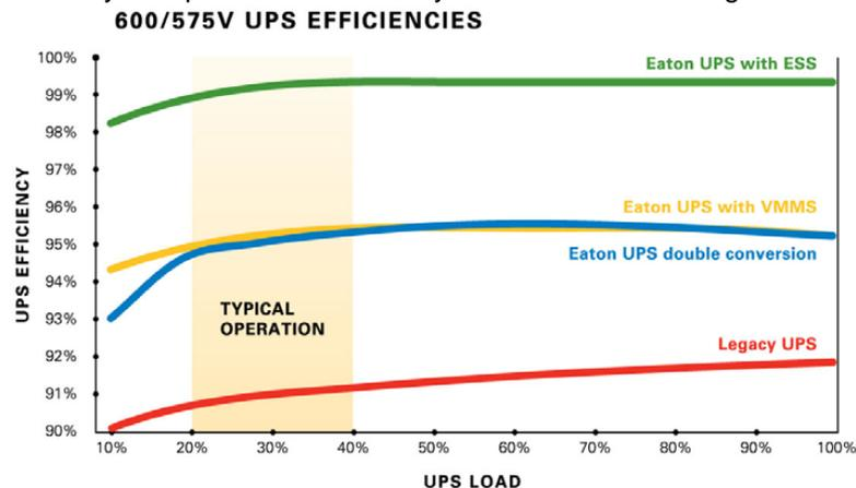
Figure 3: Efficiency gains using VMMS versus conventional mode
