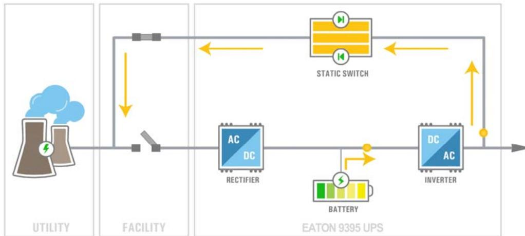
**Figure 4:** Easy Capacity Test battery discharge diagram
