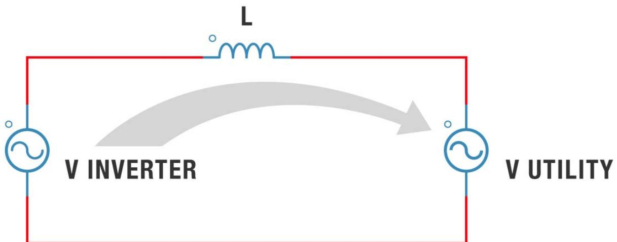
Figure 2: Power flow when inverter leads utility
