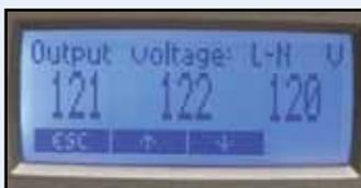
Display individual module output voltage
