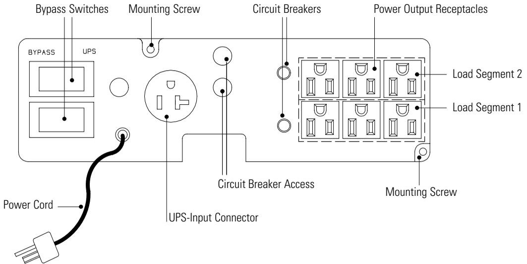
**Figure 3. PowerPass for 2000 VA, 120V UPS**
