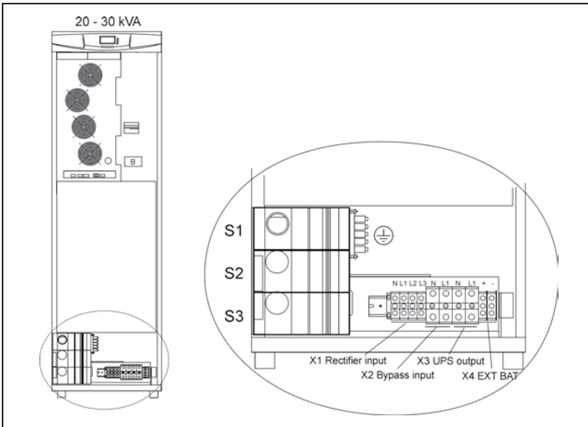
**Figure 6** Location of the power terminals. S1:Service Bypass Switch; S2:Static Bypass Input Switch; S3:UPS Output Switch. Make sure battery breaker is open and disconnect all internal battery strings before operating with the terminal X4.
