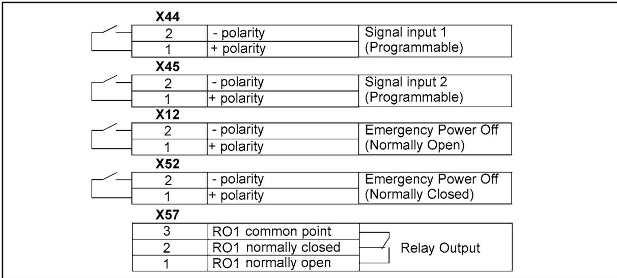
**Figure 11** External control cable connections to the UPS.
