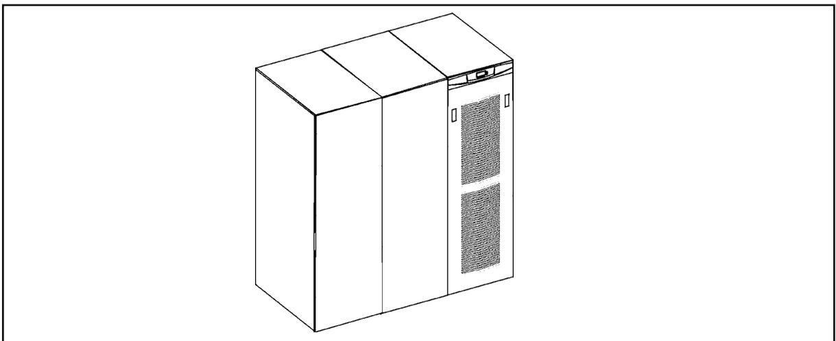
**Figure 2** UPS configuration with two External Battery Cabinets.
