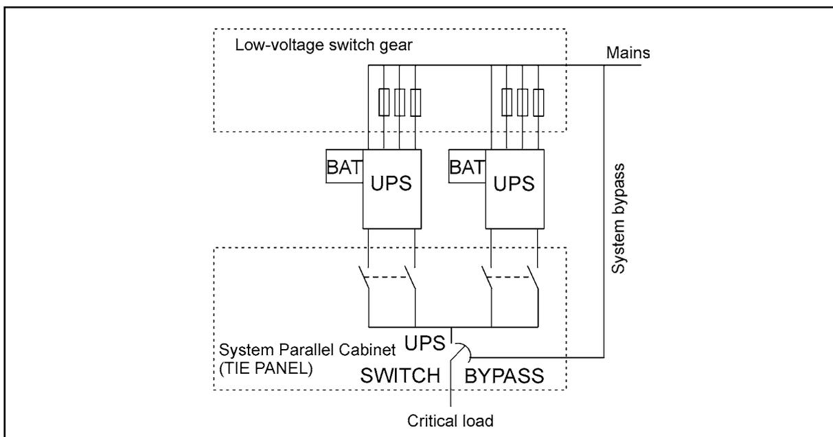
**Figure 25.** System bypass switch of the optional SPM
