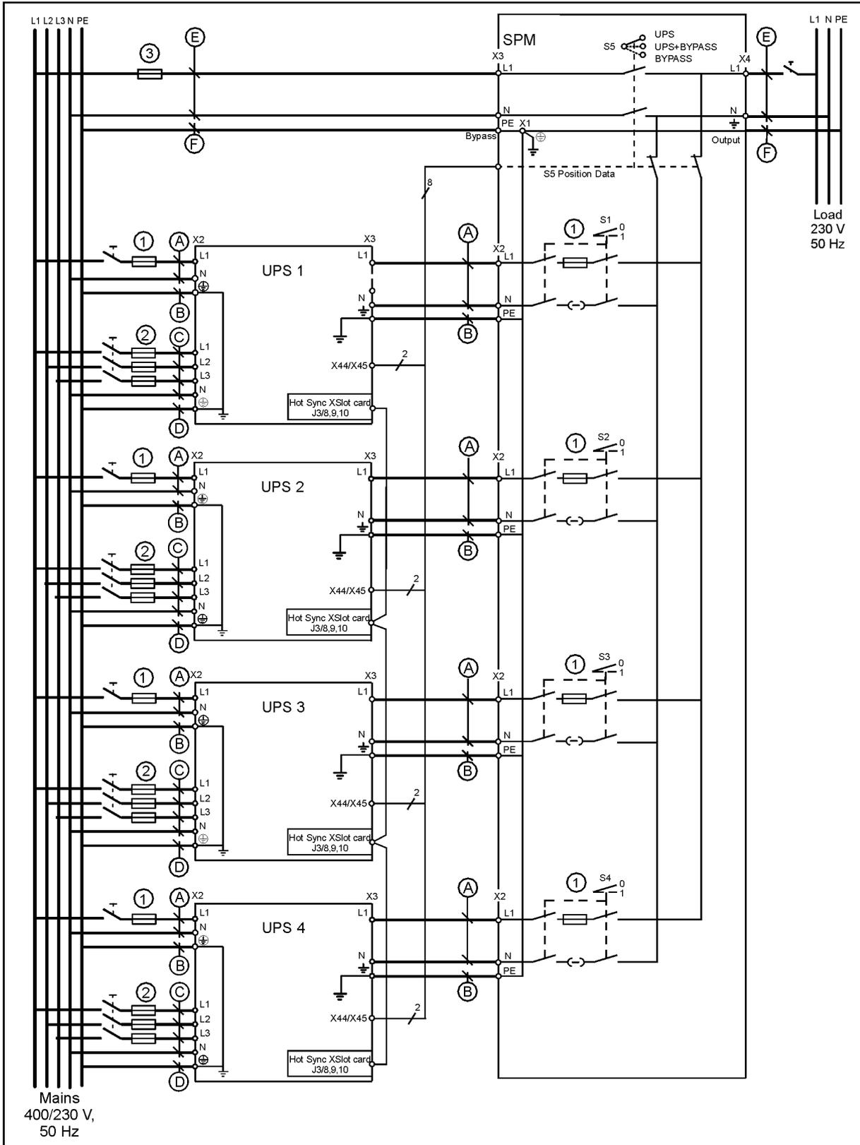
**Figure 20** Example of wiring diagram for parallel systems
