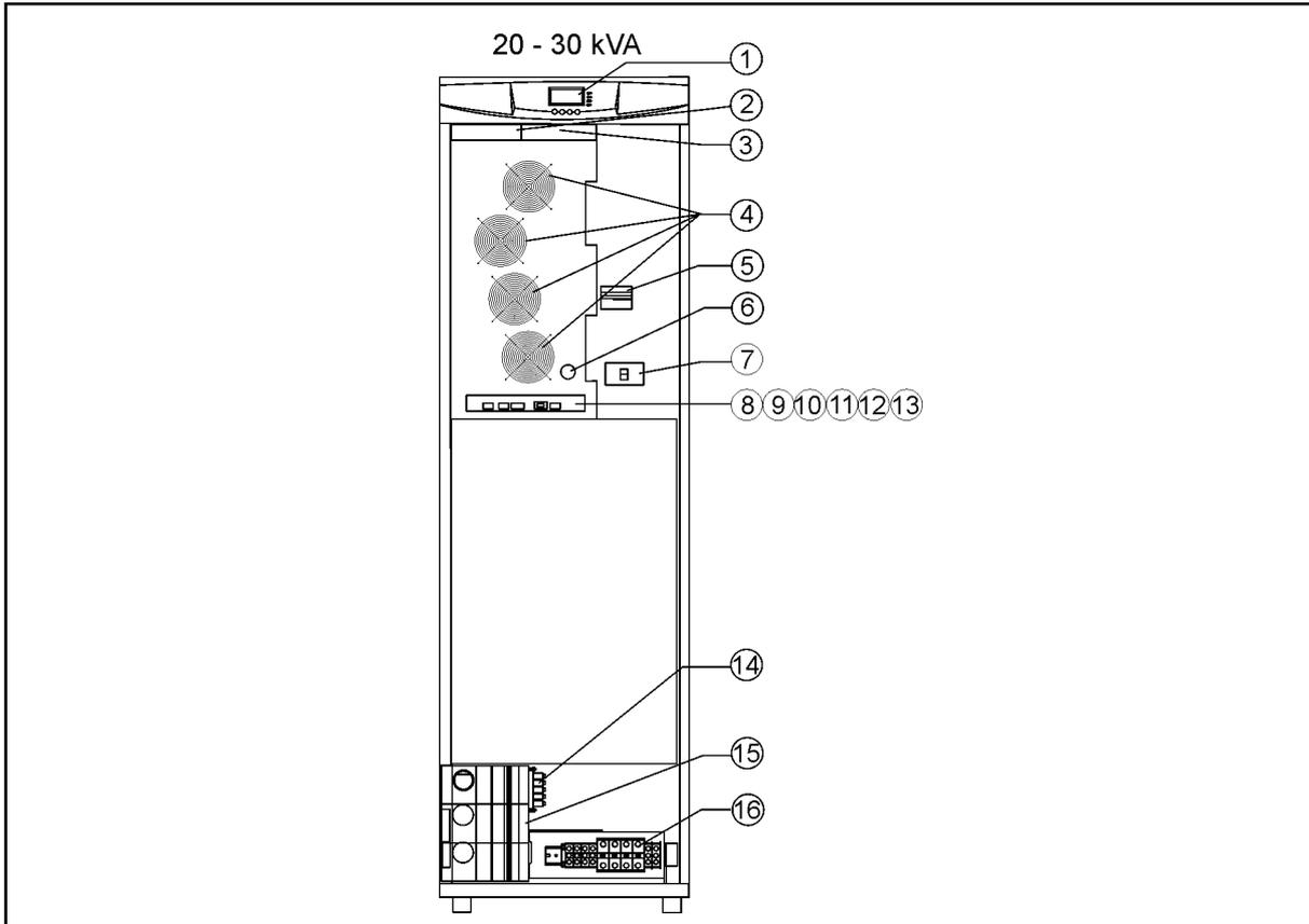
**Figure 5** Powerware 9155 20-30 kVA layout: 1:Graphical LCD; 2:XSlot-1; 3:XSlot-2; 4:Fans; 5:Input (rectifier) breaker "F2 MAINS"; 6:Battery start button; 7:Battery breaker "F1 BATTERY"; 8-13: Connectivity terminals; 14:Ground terminal; 15:MBS; 16:Power cable terminals
