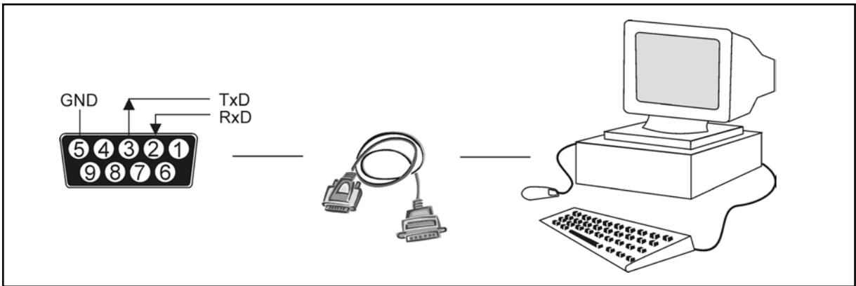
**Figure 10** Identification of the interface port pins.
