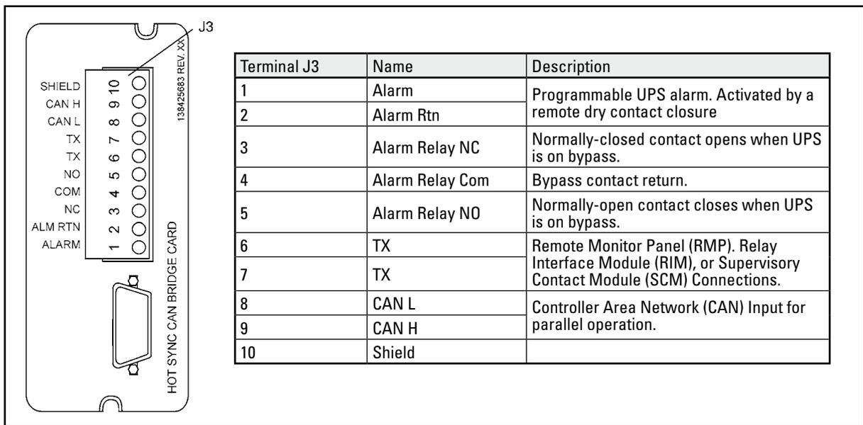
**Figure 22** XSlot Hot Sync card and terminal interface
