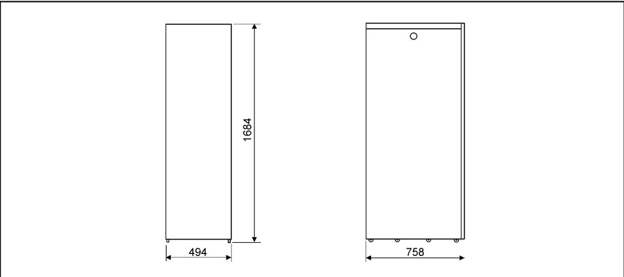
Figure 27 Dimensions of the External Battery Cabinet
