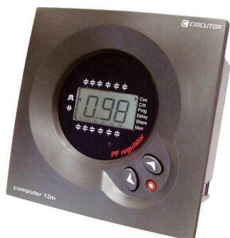
The **computer-6m / 12m** power factor regulators measure  $\cos \varphi$  in the system and regulate the connection and disconnection of the capacitors in order to correct it. Among current models there are the **computer 6m** and the **computer 12m**, with the difference being the number of relay outputs they are able to control.
